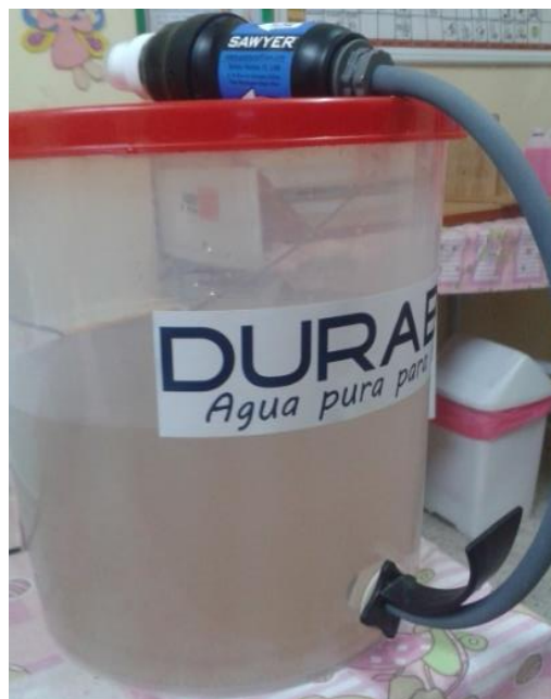
Figure 2-4. Water in the bucket obtained from the municipal tap in Independencia during the rainy season shows high turbidity.
